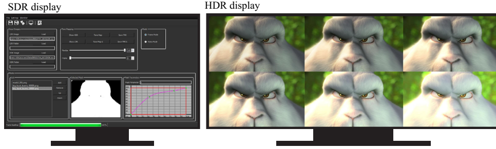
Fig. 4. This figure shows our luminance grading interface. On the SDR display, masks with values in [0, 1] can be loaded in the bottom left menu, and are displayed in the bottom-middle window. A cubic spline interface shown on the bottom right allows the user to manually input lumipaths. Different visualization options can be selected from the menu on the top. On the HDR display, users can visualize their edits in an interactive manner. To see a standard work session using our interface, we point the reader to the Supplementary material of this paper.
