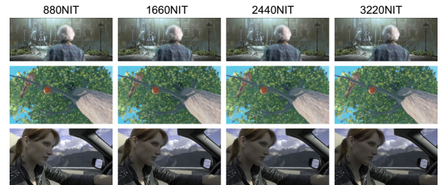
Fig. 9. Display adaptive tone mapping can be used to generate content for displays with different luminance levels, but does not allow for precise artistic control of content.
