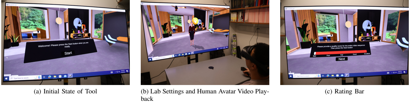
Fig. 3. (a) Initial state of the tool with a start button for users to begin the study. (b) Setup showing VR headsets, seating, and human avatar video playback on a monitor/TV. (c) Continuous rating bar displayed after each video for users to provide a quality score, with the cursor initially at the leftmost end.
