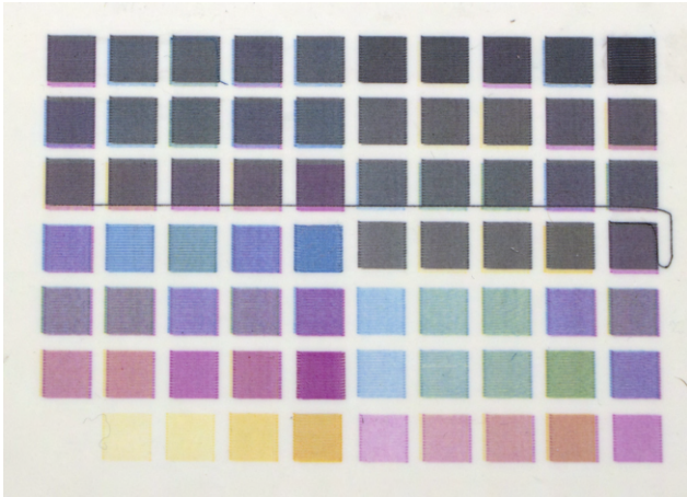
Fig. 6. The color dataset is generated by tattooing the primary inks at predefined liftoff settings in 6 \times 6 mm squares. Notably, the line tear artifact caused by the tattoo gun failing to retract during a move command has no influence on the measurements.
