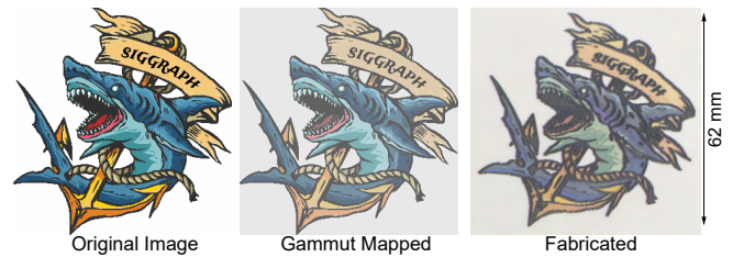
Fig. 18. Example color reproduction using our full pipeline. The input image (left) is gamut-mapped (middle) and then fabricated (right).
