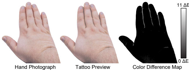
Fig. 21. The color preview shows that our tattoo machine can be used to add realistic skin-features to a bulk silicone material.
